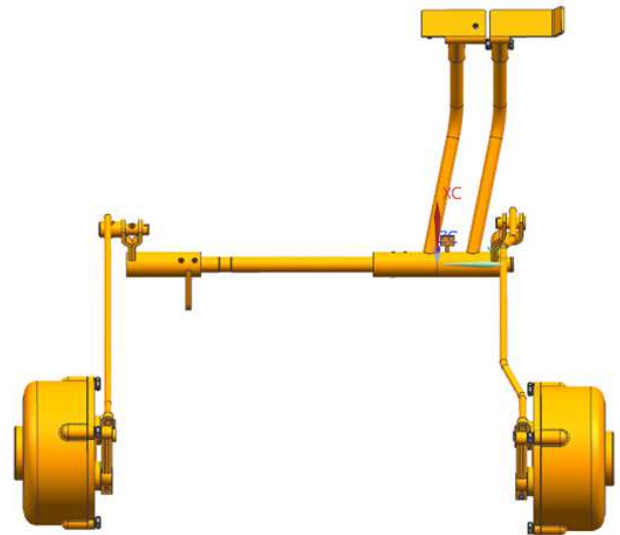
Figure 3 – The resulting parameterized model of brake
